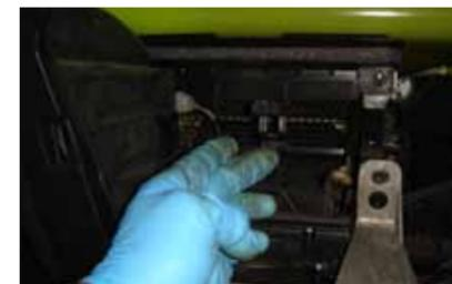
HERE I'M HOLDING THE CAGE UP TO ACCESS THE FILTER POSITION BEHIND THE GLOVE BOX.
