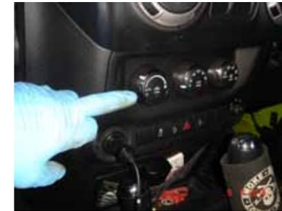
TO ACCESS THE FILTERS YOU NEED THE MOTOR RUNNING AND HIT THE RECIRCULATION BUTTON ON THE A/C SWITCH TO KEEP THE DOOR OPEN SO THAT YOU CAN ACCESS THE PAIR OF FILTERS ONCE YOU'VE POPPED THE GLOVE BOX OUT AND THE FILTER CAGE UP FROM THE BOTTOM CORNERS.
