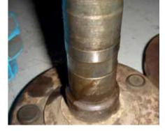
The XJ D35C rear end runs the bearing on the inner part of the axle. This axle has been chewing itself to bits for a while and you can see where the roller bearing has been chowing the face. All it's good for now is a tent peg. Twisted spline shown below.
