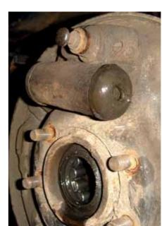
It never ends, that drum rear end on the XJ also needed wheel cylinders, they had been leaking for a long time and the rear shoes were all glazed over. Pull your drums off now and then and feel the rubber cap back. If you see fluid they're shot.
