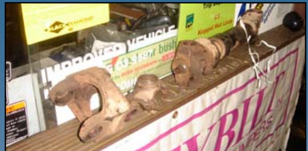
Stripped cardan joint
