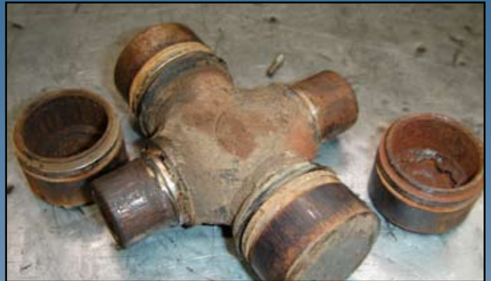
Universal joint removed from axle and caps removed show the wear and missing rollers
