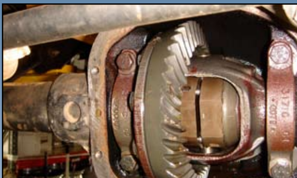
Chipped teeth on the crownwheel
