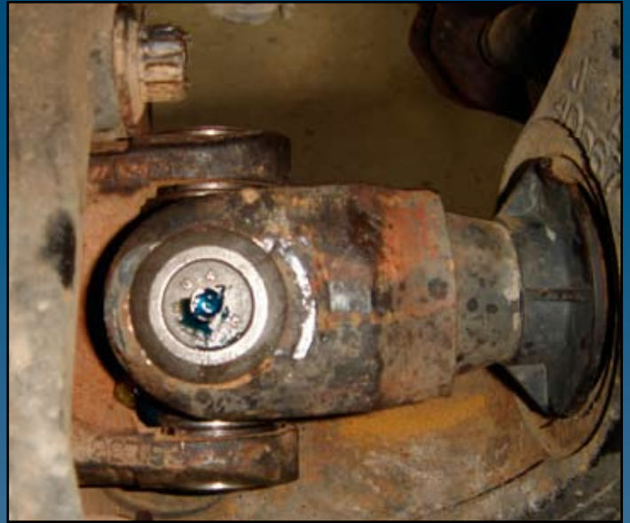
Greasable universal joint fitted to front axle
