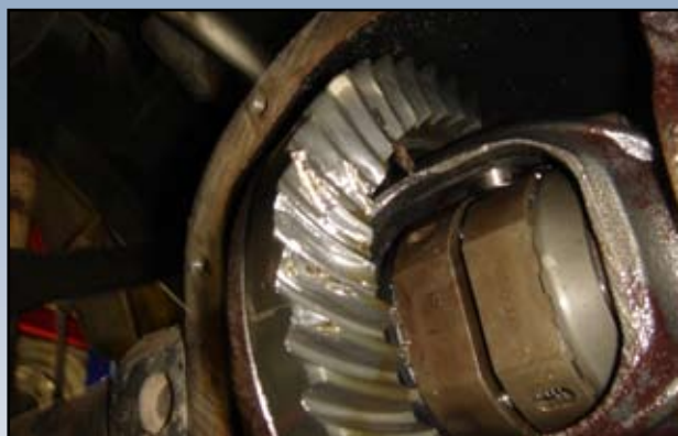
Chipped teeth on the crownwheel
