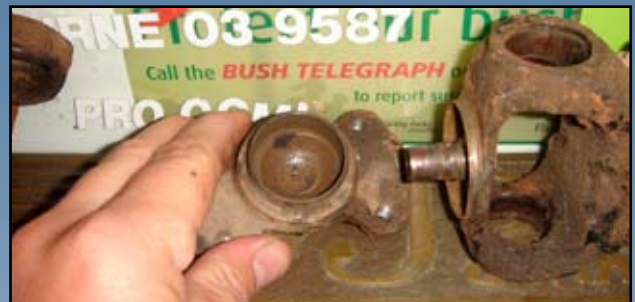
Stripped cardan joint
