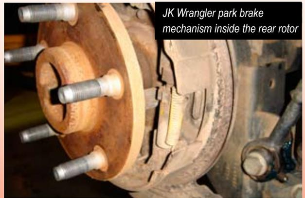
JK Wrangler park brake mechanism inside the rear rotor
