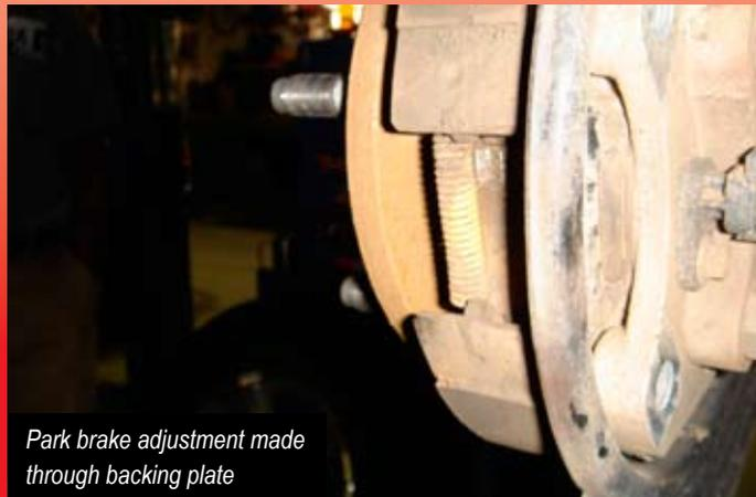
Park brake adjustment made through backing plate
