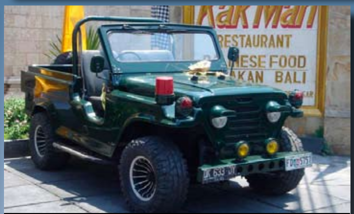
This must have been a Nissan G60 once, now it has a fibreglass body and a Mutt M151 grille. The red lamps were used by police but are also simply used as decoration. It has a Fremantle Dockers license plate.
