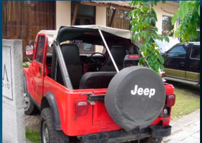
A run down 1983 CJ7 parked and forgotten running YJ axles and wheels
