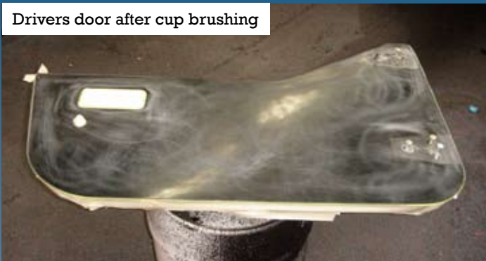
The internal area after cup brushing
