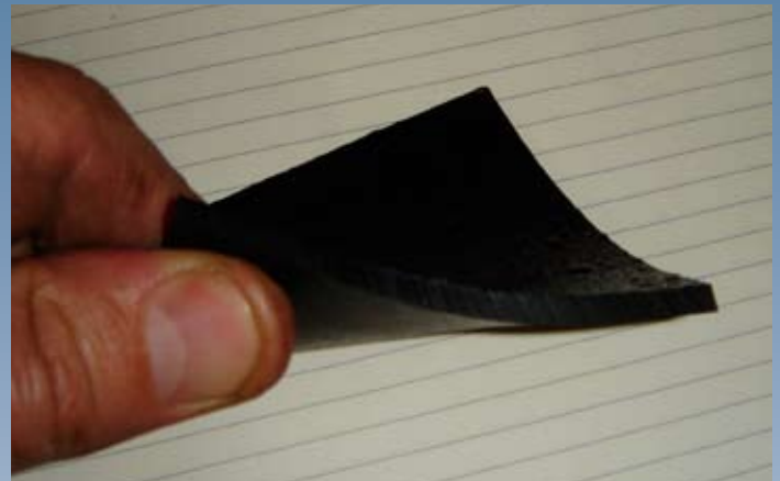
A sample of rhino tuff stuff, it's flexible, can be applied up to 5mm thick and is literally bullet proof! Various armies around the world use it to bomb-proof their vehicles and even make fuel tankers bullet proof. Technically a bullet will pass through the surface but it will close over the hole stopping the tanker from leaking when shot at.
