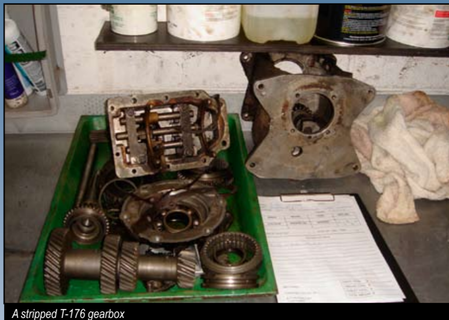
A stripped T-176 gearbox
