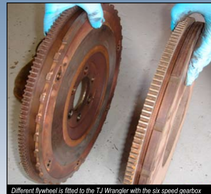
Different flywheel is fitted to the TJ Wrangler with the six speed gearbox
